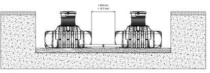
GARANTIA special crown bit. It must be ensured that the distance between the tanks is at least 500 mm (19.7 inch). The pipes must project at least 200 mm (7.9 inch) into the tanks.
