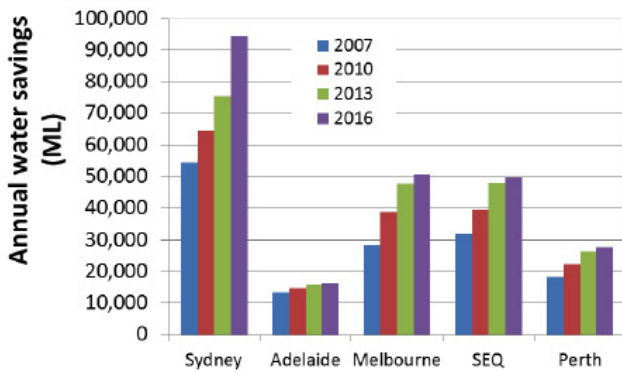
Figure 8: Annual water savings from water efficient appliances and rainwater harvesting for the Sydney, Adelaide, South East Queensland and Perth urban regions
